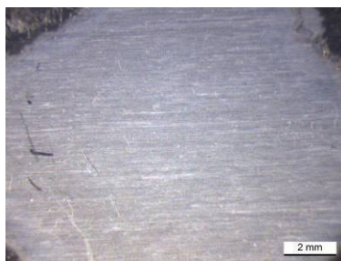
Sample 2. Square surface after electrochemical anodizing, 10 times magnification in a microscope.
