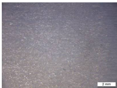
Sample 2. Drop of chemical anodizing, 10 times magnification in a microscope.
